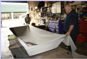
First we do the headliner on the new roof
