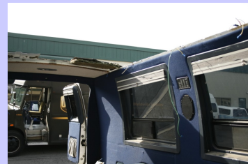
Old roof comes off
